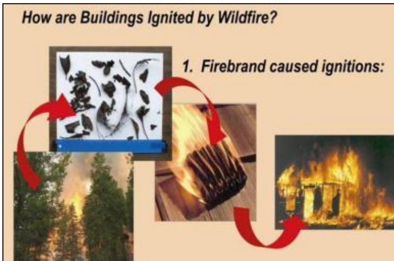
Figure 6. Firebrand caused ignitions: burning embers are carried ahead of the fire front and alight on vulnerable building surfaces.
