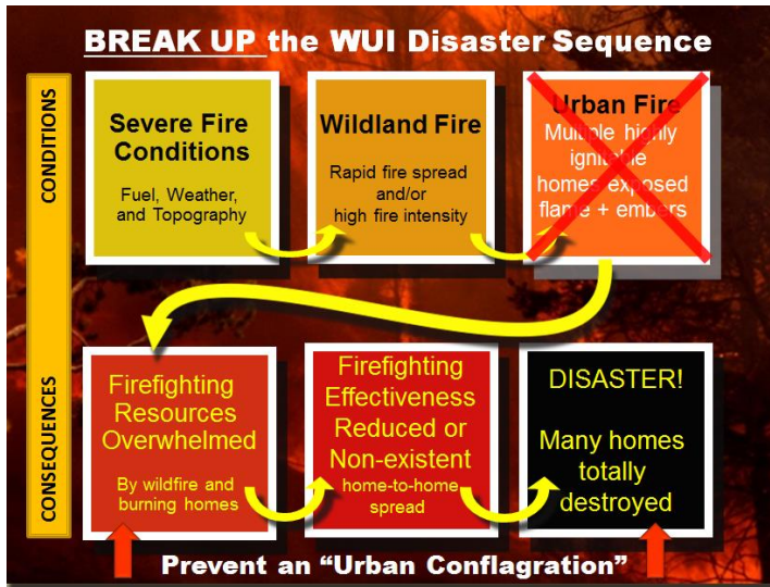
Figure 3. Wildland/urban interface disaster sequence. 89 It is possible to break up the disaster sequence by decreasing the number of highly ignitable homes exposed to embers, therefore reducing the number of homes ignited and removing the consequences of multiple structures lost.
